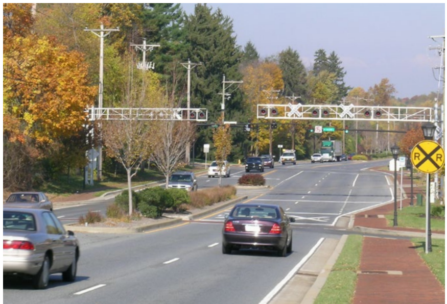
Streetscaping in Centreville, New Castle County, Delaware includes landscaped medians, street trees, brick sidewalks, and pedestrian scaled lighting.
